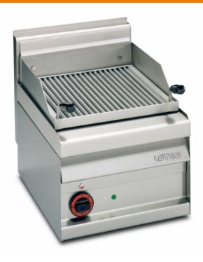
Construction - Fabricated using CrNi 18/10 AISI 304 grade Stainless Steel Scotch-Brite Satin polish Finish, incorporating 1mm thick worktop, rounded edges, chromed details and rear splash back. Model -Professional Electric Grill. Fitted with water compartment and special reflective system to optimise heat, Removable liquid containers. Maintenance - All serviceable parts are accessible by the easy removal of front control panel. Fittings - Appliance is supplied with adjustable feet.
